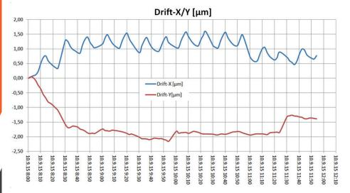
Focal spot movement of XWT-160-TCNF. Parameters: 100 kV, 1 Watt target power, submicron mode, centering and filament-adjust every 30 minutes
